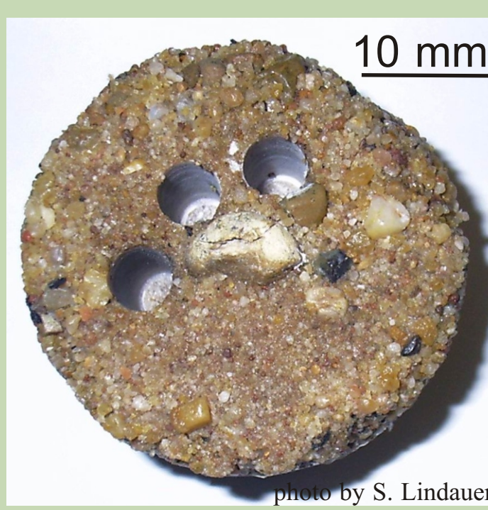
Fig. 9: Alluvial sand from Mauer embedded in resin (with 3 drilling holes).
