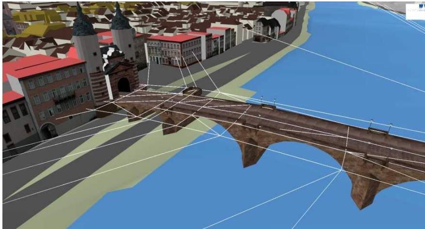
Fig. 6: For bridges and tunnels a second surface model is used in addition to the usual terrain (here rendered as wireframe model).
