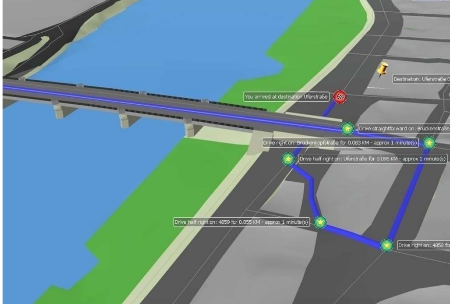
Fig. 5: Example for routing with our 3D routing service at several streets levels: route crossing underneath a bridge. The network is shown as thin lines.
