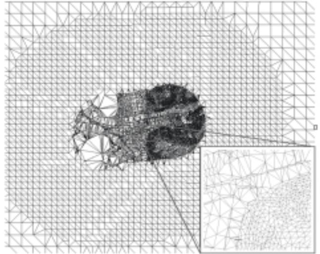
**Figure 10: Multi-Resolution-DEM generated dynamically to suite a specific tour (TIN representation)**
