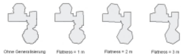
Figure 13: Results of different values for generalization of building footprints.
