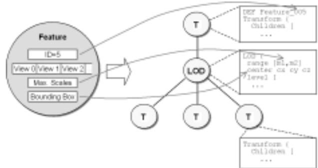
Figure 8: The export of different geometric representations of the same (VR)-Feature to different LODs in VRML
