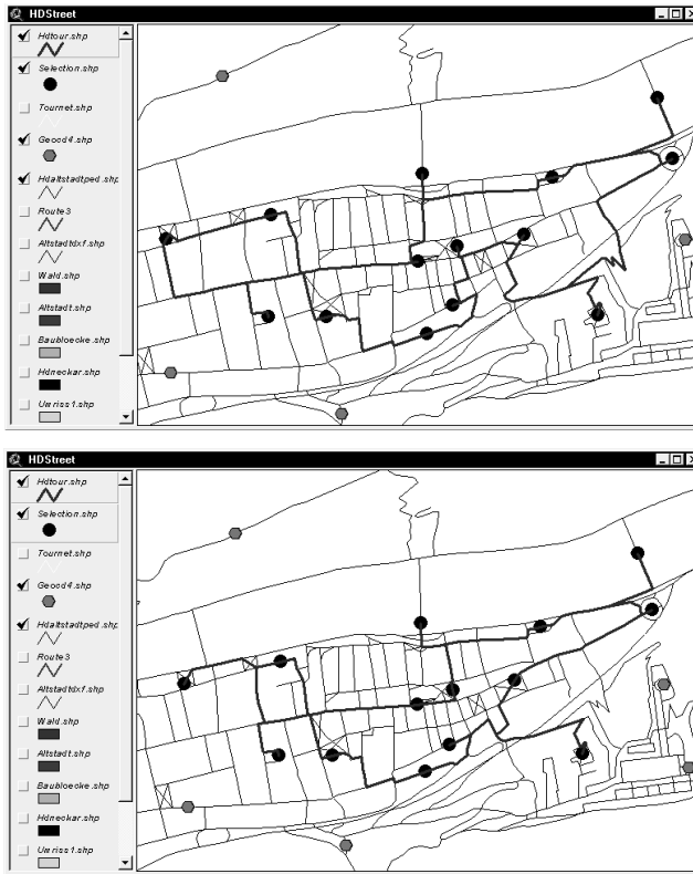
Fig. 3. Calculated tours for passenger with high preferences against noise and smoke versus high preferences for attractive areas.
