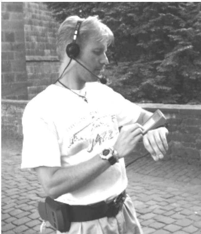
Figure 3. The Deep Map system in mobile use. The Tourist has a head set for natural language interface, a display on his arm and a wearable computer mounted on his belt (Xybernaut MAIV pentium system).
