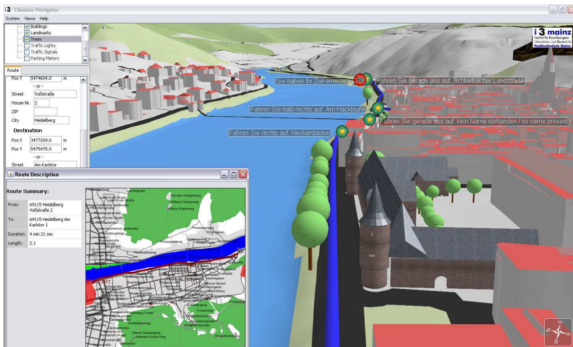
Figure 7: Representation of a requested route and within the respective 3D city-model along with route instructions
