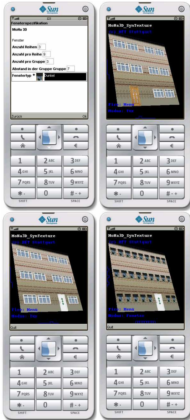
Figure 6: Upper left: User Interface to specify the pulse function for window layer, upper right: the facade generated by this pulse function with an additional layer to position a door; lower left – similar with another position of the door; lower right – variation of the window layer pulse function.
